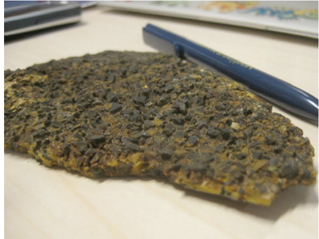
Figure 12. A non-slip but highly abrasive flooring material used on some ships.
